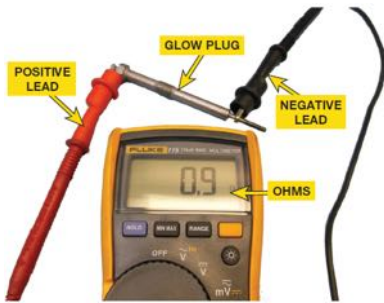
FIGURE 10–14 ohmmeter shows a resistance of 0.9 ohms which is normal for most glow plugs that usually have a specification of 0.6 to 6.0 ohms. Check service information for the exact resistance specification for vehicle being tested.
