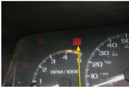
FIGURE 10-12 The Wait-To-Start Light is controlled by the powertrain control module and is illuminated during the time the glow plugs are heating.
