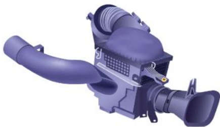
FIGURE 10-2 The air filter housing contains two air inlets. The inlet in the fender is for normal operation and the ram air inlet faces the grille opening.
