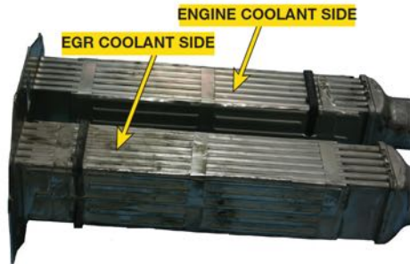
FIGURE 10–16 The EGR cooler lowers the exhaust gas temperatures, allowing it to absorb more combustion chamber heat.
