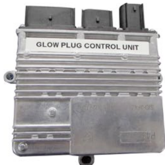
FIGURE 10-11 This glow plug control module example is from a Nissan Titan equipped with a 5.0 liter Cummins engine. The module controls the glow plugs based on messages received from the powertrain control module on the high speed CAN Bus network.
