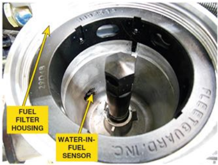
FIGURE 12-10 water-in-fuel sensor uses electrical conductivity to sense the water in the fuel. If the conductivity is above a specific level, the warning lamp on the dash is illuminated.
