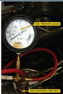
FIGURE 12-11 low-pressure fuel system can be tested with a traditional fuel pressure gauge and the required adapters.
