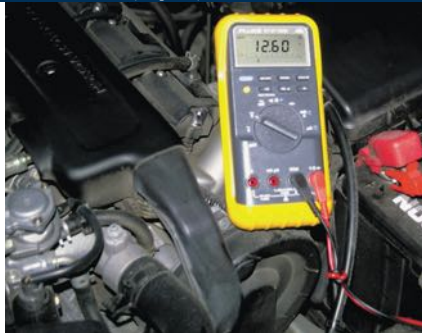
FIGURE 17-14 digital multimeter set to read DC volts is being used to test the voltage of a vehicle battery. Most multimeters can also measure resistance (ohms) and current flow (amperes).
