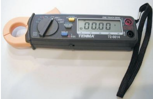
FIGURE 17-36 typical mini clamp-on-type digital multimeter. This meter is capable of measuring alternating current (AC) and direct current (DC) without requiring that circuit be disconnected to install meter in series. The jaws are simply placed over wire and current flow through circuit is displayed.
