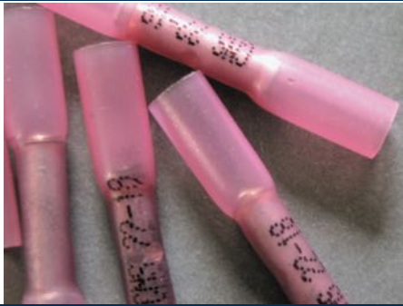
FIGURE 17-45 typical crimp-and-seal connector. This type of connector is first lightly crimped to retain ends of wires and then it is heated. The tubing shrinks around wire splice, and thermoplastic glue melts on inside to provide an effective weather-resistant seal.
