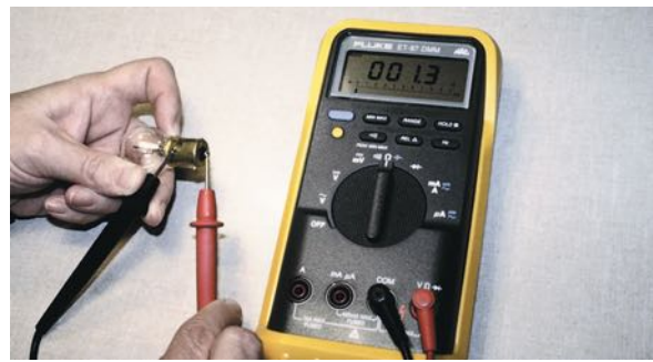
Figure 17-31 Using a DMM set to read ohms ( \Omega ) to test this light bulb. Meter reads resistance of filament
