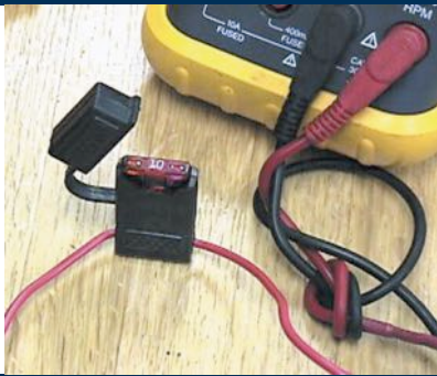
FIGURE 17-34 Note blade-type fuse holder soldered in series with one of meter leads. A 10-ampere fuse helps protect internal meter fuse (if equipped) and meter itself from damage that may result from excessive current flow if accidentally used incorrectly.
