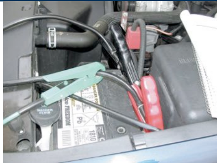
FIGURE 17-35 inductive ammeter clamp is used with all starting and charging testers to measure the current flow through the battery cables.
