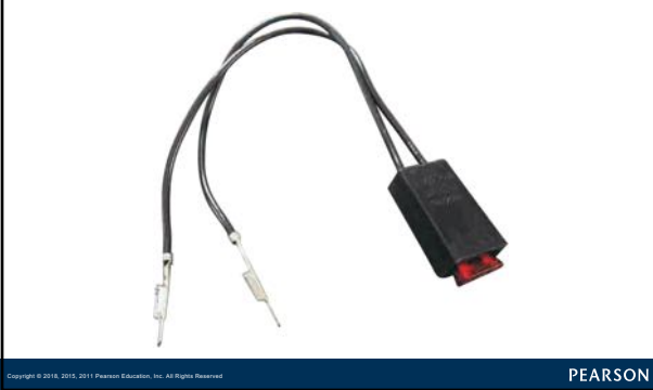
FIGURE 17-25 A technician-made fused jumper lead, which is equipped with a red 10-ampere fuse. This fused jumper wire uses terminals for testing circuits at a connector instead of alligator clips.
