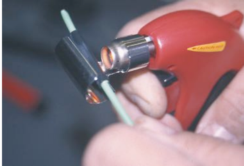
FIGURE 17-44 butane torch especially designed for use on heat shrink applies heat without an open flame, which could cause damage.
