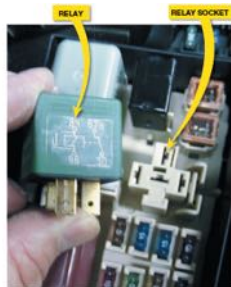
FIGURE 17-49 typical relay showing schematic of wiring in relay.
