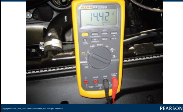
FIGURE 17–29 Typical digital multimeter (DMM) set to read DC volts.
