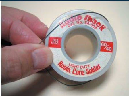
FIGURE 14-41 Always use rosin-core solder for electrical or electronic soldering. Also, use small-diameter solder for small soldering irons. Use large-diameter solder only for large-diameter (large-gauge) wire and higher-wattage soldering irons (guns).
