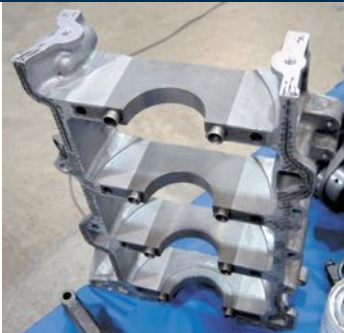
FIGURE 2-9 (A) bedplate is a structural part of the engine which is attached between the block and the oil pan and supports crankshaft.
