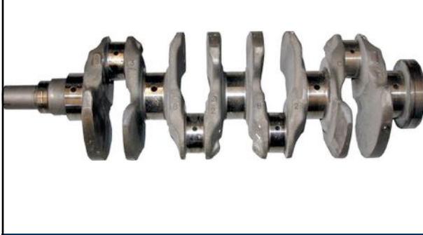
FIGURE 2-18 fully counterweighted four-cylinder crankshaft with five main bearings.
