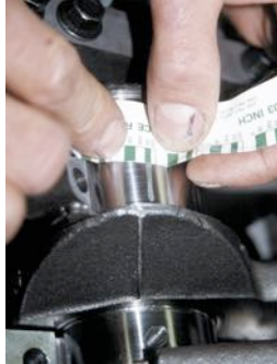
FIGURE 2-30 width of plastic gauging strip determines oil clearance of the main bearing. Alternate method of determining oil clearance includes careful measurement of crankshaft journal and bearings after they are installed, and the main housing bore caps are torqued to specifications.
