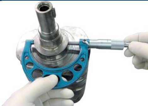
FIGURE 2-22 All crankshaft journals should be measured for diameter as well as taper and out-of-round.
