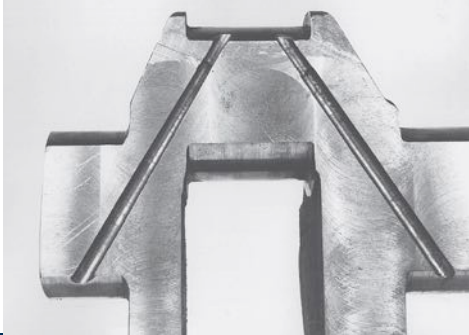
FIGURE 2-16 Crankshaft sawed in half, showing drilled oil passages between the main and rod bearing journals
