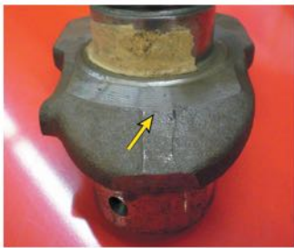
FIGURE 2–14 Wide separation lines of a forged crankshaft..
