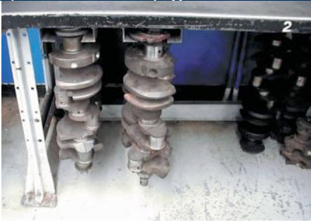
FIGURE 2-24 Crankshafts should be stored vertically to prevent possible damage or warpage. This clever bench-mounted tray for crankshafts not only provides a safe place to store crankshafts, but is also out of way & cannot be accidentally tipped.
