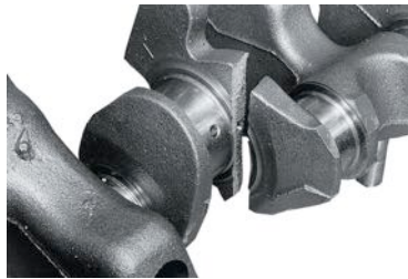
FIGURE 2-19 crankshaft broken as a result of a defective torsional vibration damper.
