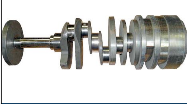
FIGURE 2-15 billet crankshaft showing how it is machined from a solid chunk of steel, usually 4340 steel, at the right and the finished crankshaft on the left.
