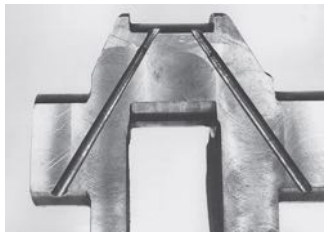
FIGURE 2-16 Crankshaft sawed in half, showing drilled oil passages between the main and rod bearing journals Larger in next slide
