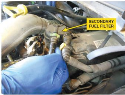
FIGURE 22–15 connector tabs are depressed to release them from the fuel filter.
