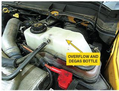
FIGURE 22–3 overflow and Degas bottle located under hood on driver’s side.
