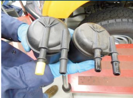
FIGURE 22–16 new filter is on left and old filter is on right. Dispose of old filter according to federal, state, and local laws. (SECONDARY)
