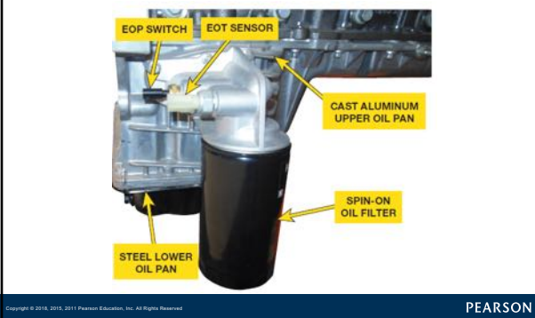
FIGURE 22-4 oil filter used on 6.7 Power Stroke is a spin-on type. Oil pan was updated for 2012 model year with stamped steel lower pan with conventional plug instead of plastic (composite) pan used with plastic drain plug on 2011 model year version.
