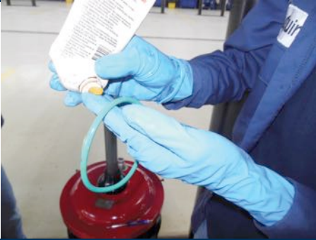
FIGURE 22–14 Lubricating the O-ring with grease will allow the housing to move freer when the housing is being rotated back into the DFCM.
