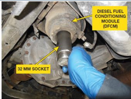
FIGURE 22–12 Use 32 mm socket with a ratchet to loosen filter housing. After loosening, housing can often be removed by hand, rotating it counterclockwise.
