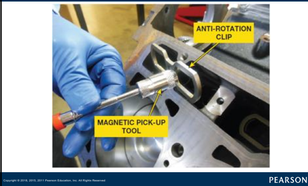
FIGURE 23–6 (b) To keep valve lifters from rotating in their bores, an anti-rotation clip is used that allows lifters to move up and down freely.
