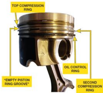
FIGURE 23-4 piston has 4 grooves for 3 piston rings, but one of 3 grooves is used as heat dam & often referred to as “empty piston ring groove”.
