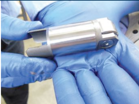
FIGURE 23–6 (a) Duramax diesel engine uses large diameter roller solid (non-hydraulic) valve lifters.
