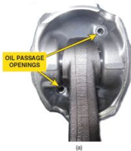
FIGURE 23-5 (a) openings on underside of piston are designed to allow engine oil to flow to head of piston.
