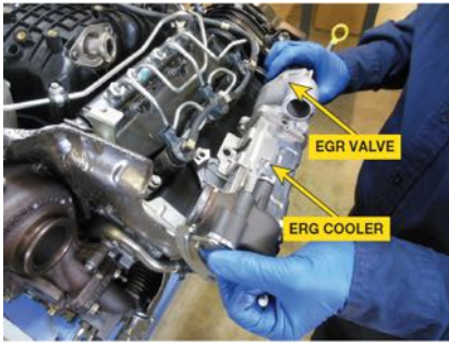
FIGURE 25–20 EGR valve is mounted on end of EGR cooler. Together they reduce level of NOx emissions by controlling flow and temperature of EGR gasses.
