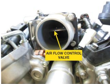
FIGURE 25–21 air flow control valve creates negative intake air pressure that increases flow of EGR gasses.
