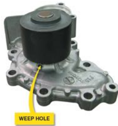
FIGURE 5-16 bleed weep hole in the water pump allows coolant to leak out of the pump and not be forced into the bearing. If the bearing failed, more serious damage could result.
