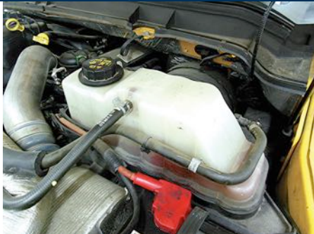
FIGURE 5-13 Some vehicles, such as this FORD F-250 pickup truck equipped with a 6.7 liter power stroke diesel engine, use an expansion tank, which is located at the highest level of the cooling system.
