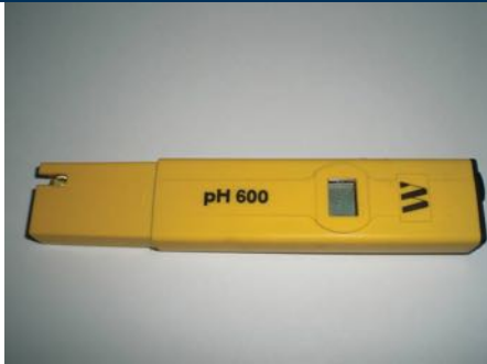
FIGURE 5-30 meter that measures actual pH of coolant can be used for all coolants, unlike many test stripes that cannot be used to test the pH of red or orange coolants.
