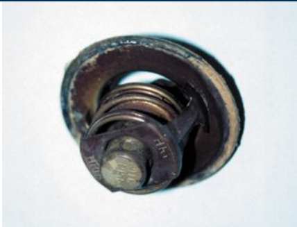
FIGURE 5-5 thermostat stuck in the open position caused the engine to operate too cold. If a thermostat is stuck closed, this can cause the engine to overheat.
