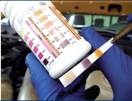
FIGURE 5-28 Test strip can be used to determine pH and percentage of glycol of coolant. Percentage of glycol determines freezing and boiling temperatures, as shown on bottle that contains test strips.
