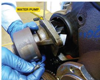
FIGURE 5–14 Water pump from front of Cummins 6.7 liter diesel engine.
